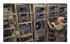
In 1948 the world's first storedprogramme electronic digital computer was born at the University of Manchester – nicknamed the 'Baby'. It stored 2048 bits, compared to the millions of bits on today's computer chips.
