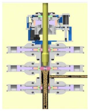
Fig. 4. Coupler device used in the continuous circulation system <sup>[13]</sup>
