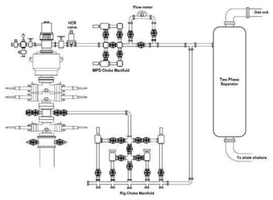
Fig. 3. Rig up for CBHP applications. [12]
