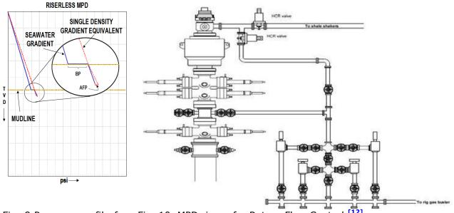
Fig. 9.Pressure profile for Fig. 10. MPD rig up for Return Flow Control <sup>[12]</sup> drilling dual gradient without a riser <sup>[16]</sup>
