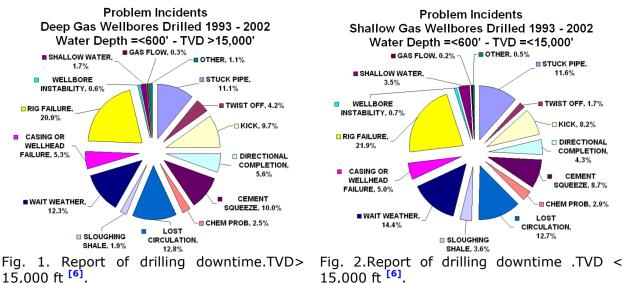
MPD can solve a large percentage of the problems the database lists, especially those that are caused by wellbore pressure deviating out of the pressure gradient window during drilling operations. Table 1 shows the NPT from Fig. 1 that could be reduced by using MPD <sup>[6]</sup>.
