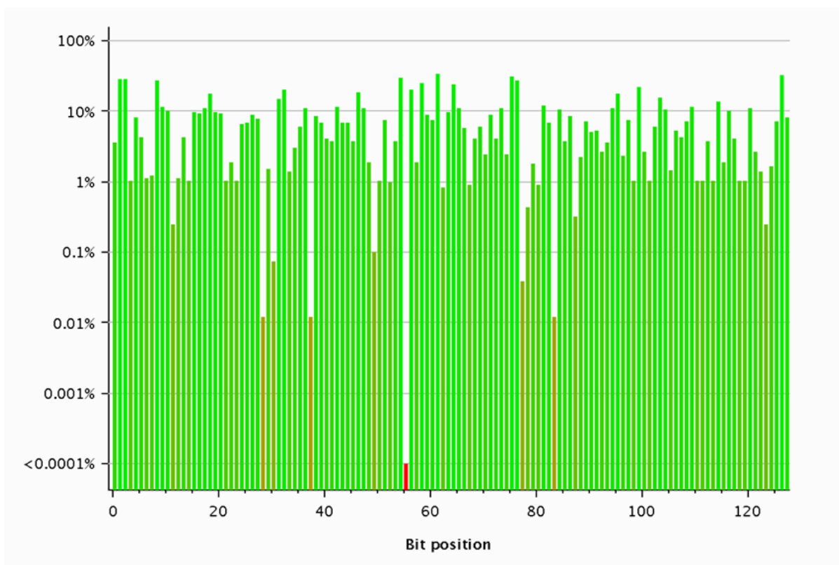
Figure 4: Chart indicating the degree of confidence in the randomness of the sample at each bit position from the cookie obtained from the ClientCompany application
