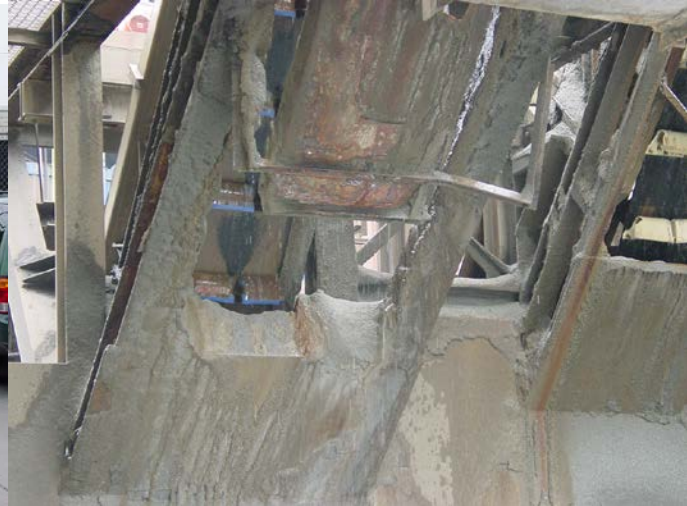
Figure 8. Wind Protection for Unloading of Fine PM
