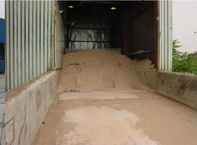
Figure 8. Wind Protection for Unloading of Fine PM
