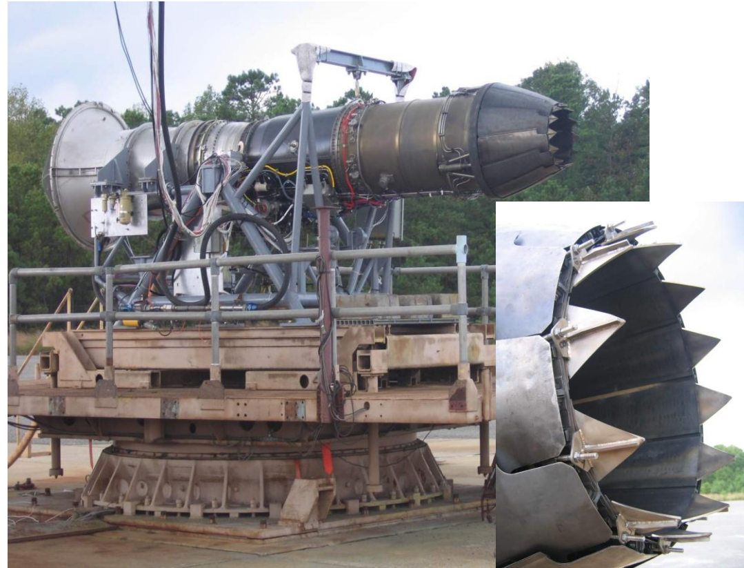
Prototype Chevrons being tested on the F/A-18 engine by ONR/GE at Naval Air Warfare Center Aircraft Division, Lakehurst, 9/07
