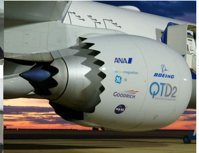
Flight Test with Chevrons on GE-90-115B
