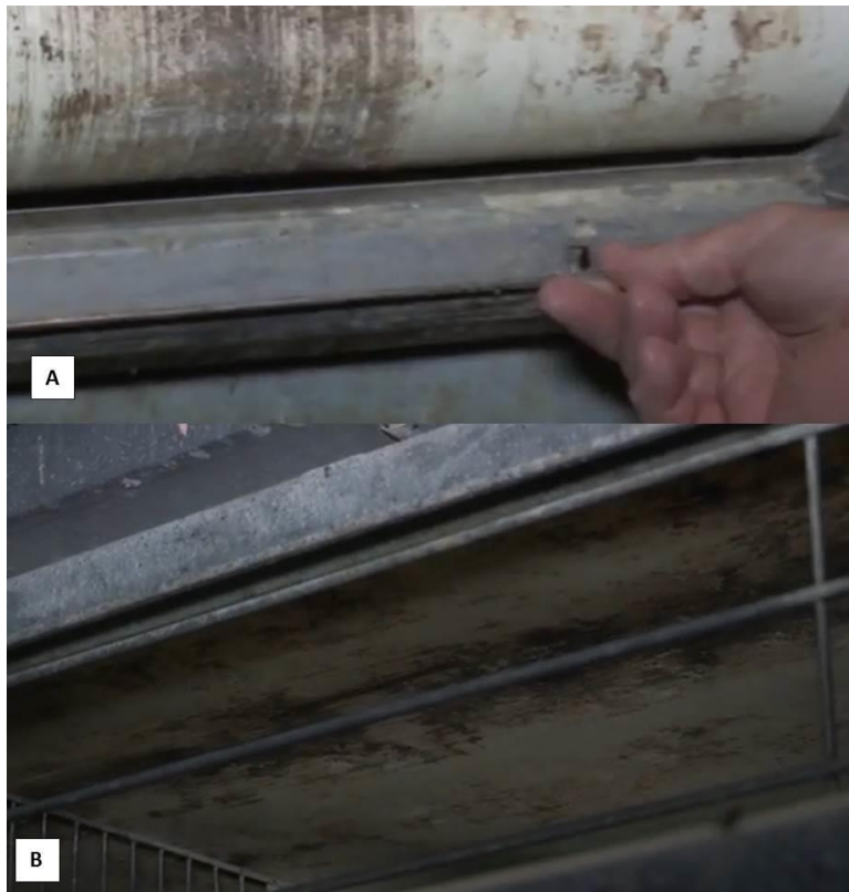
Figure 12. Example of a manure belt in use during pullet rearing. The scraper removes most, but not all the manure (A) and is not equipped to remove microscopic organisms, such as Eimeria . In a multi-tier conventional cage system, the manure belt acts as a roof for the tier below (B). Pullets in lower tiers may have access to Eimeria from the manure belt, especially when they are tall enough to peck at the belt. (Picture Credits: Guy Kostrey, Scenescape Productions)
