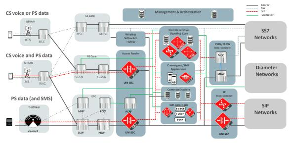
Figure 4: Next Generation Robust Signaling Infrastructure
