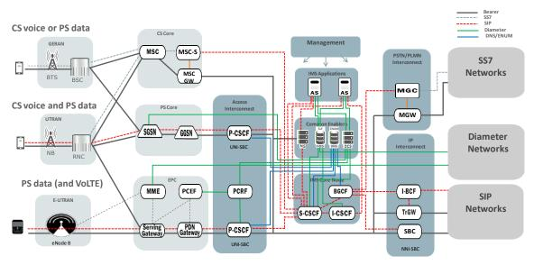
Figure 3: Traditional Signaling in LTE and IMS Networks
