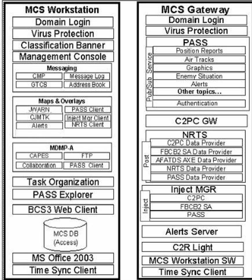
Figure 1-1 Workstation and Gateway assets
