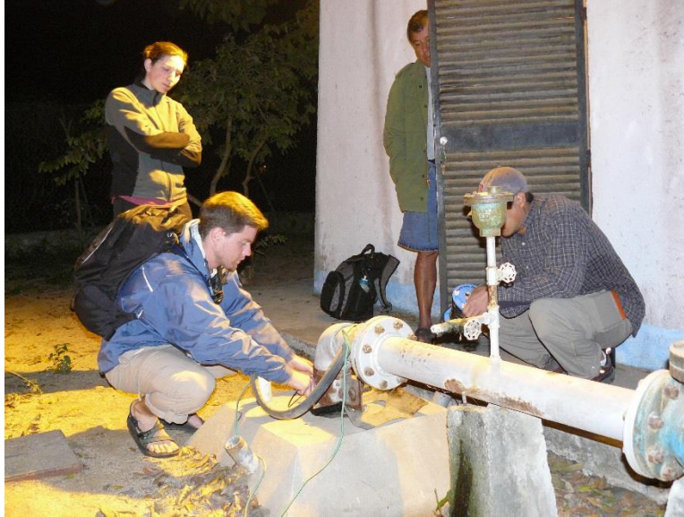
Figure 26. Conducting an aquifer performance test on a well in a rural community in Mexico.
