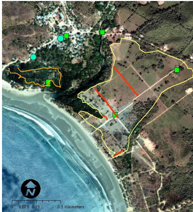
Figure 20. Constructed features to allow passage over water or to move water out of the community or off of the agricultural lowland. Blue circles are surface water runoff from the community observed in the dry season; green squares are bridges and culverts; red lines are ditches; and the orange line is a proposed trail which will include an improved bridge. The yellow line delineates the agricultural lowland and is provided for reference.
