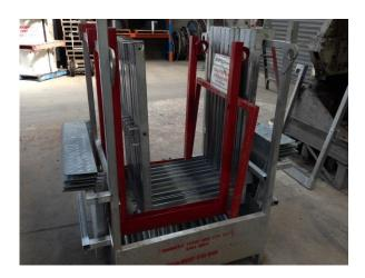
Your scaffold will come in a stillage looking like this. Typically there are 2 sections of scaffold to each section of outer drum. ie; 12 brackets, 12 floor plates, 24 balustrade rails and 1 tensioning strap.
