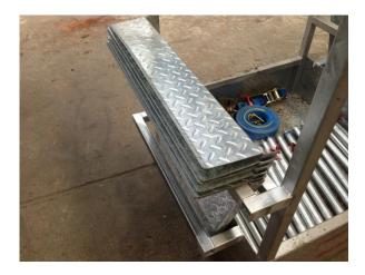
Take one of the floor plates from its cradle, located on the outside of the stillage.
