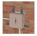
The protection cover protects the inner parts of the box during installation procedures.
