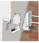
Plaster the wall or lay the tiles right up to the edges of the protective mask.
