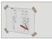
Make the reference marks using the special template and drill the wall.
