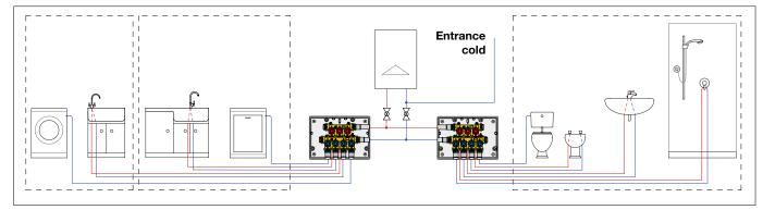
Independent system: multi-floor home (boiler with storage and recirculation)
