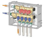
Installation with tee for recirculation circuit and with passing through outlet.
