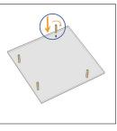
Screw the pins to the rear of the plate.
