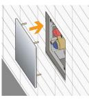
Fasten the aesthetic cover plate to the cylindrical guides.
