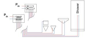
Manifold with individual shut-off valves
