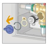
Cartridge for main shut-off valves
