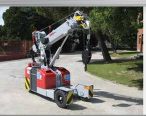
New Valla 25E is the light weight precision pick and place crane. It can handle high-value products such as glass and cladding panels. It moves easily between floors and improve installation timing and better safety for operators.
