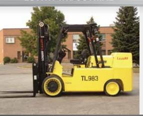
Cushion tire industrial workhorse with capacities from 18,000 lbs. to 45,000 lbs. Propane or Diesel clean-burn engines with electronic transmission control.
