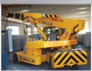
The Valla 120E is a precision movement mobile pick and carry crane. It's lifing capacity of 12 tons (24,000 lbs) makes it ideal for heavy and delicate picks.
