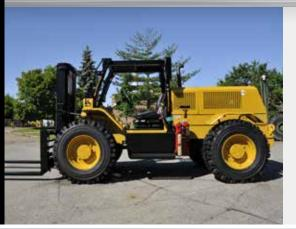
Compact models designed for applications limited on space with capacities up to 10,000 lbs. and various drivetrains available.
