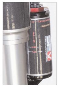
shock and what the pump is reading. This is all normal procedure when adjusting the air spring pressure. After removing the pump, be sure to reinstall the Schraeder
