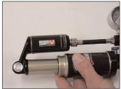
usually a 10-15 psi difference between what was in the shock and what the pump is reading. This is normal procedure when adjusting the SPV shock pressure. After removing the pump, be sure to reinstall the Schraeder valve cap. If the shock does not dampen properly after pressurizing, the air pressure was lost during pump removal as a result of a worn or malfunctioning pump fitting o-ring. Do not ride the bike until the shock is pressurized.
