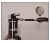
only the air left in the pump itself and not from the shock. This does not affect your pressure setting in the shock. Likewise, when you install the pump, the shock will fill the pump and reduces the registered pressure previously installed in the shock. This usually is a 10-15 psi difference between what was in the
