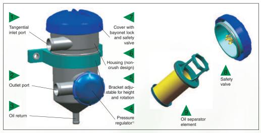
Fig. 1: Components with example of ProVent® 200
