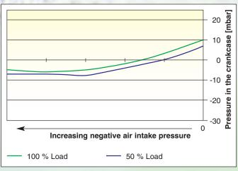
Fig. 3: Pressure adjustment curve (ProVent® 200)
