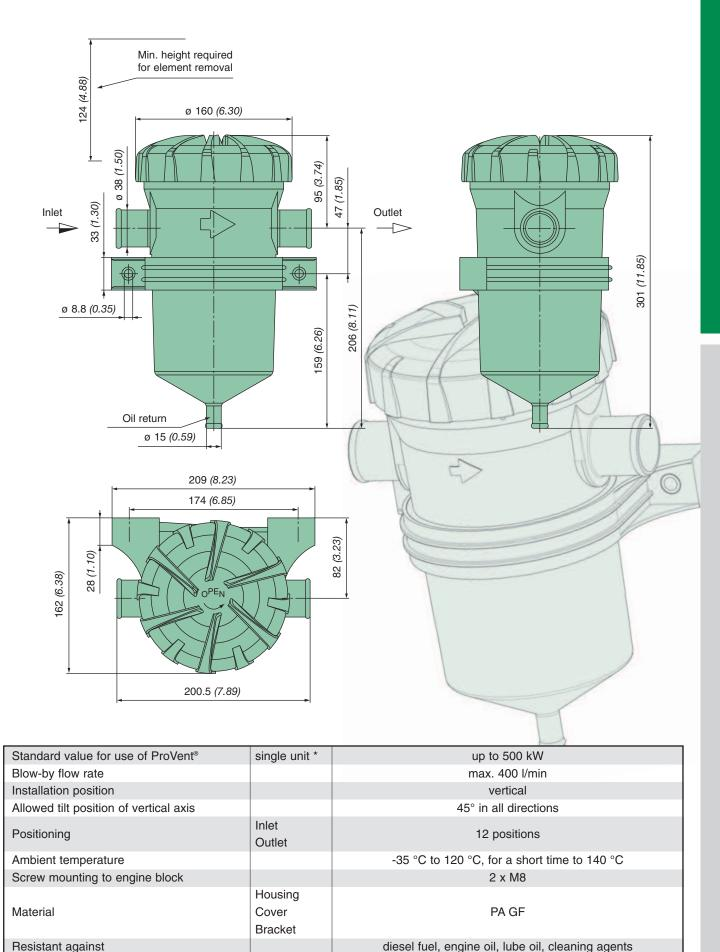
$<sup>^{\</sup>star}$  Use of two ProVent  $\!\!^{\circ}$  of the same type in parallel possible
