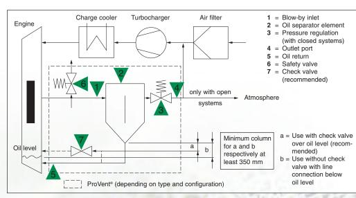
Fig. 2: Diagram of closed and open crankcase ventilation
