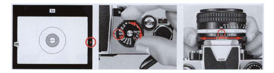
Position your main subject at the centre of the field of view inside the viewfinder. Then turn the shutter speed dial and/or lens aperture ring until the LED lamp for the symbol for correct exposure **O** lights up.
