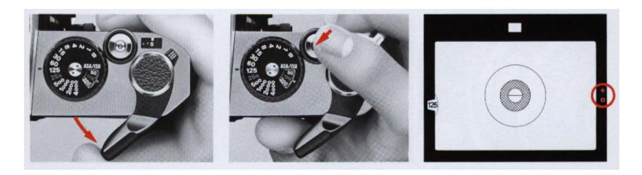
Pull out the film advance lever to unlock the shutter release button. This lever doubles as a shutter release lock.
