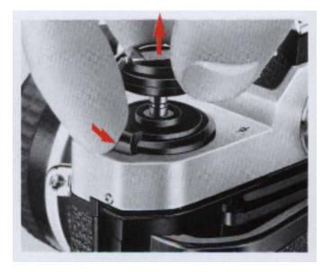
Push the camera back lock lever counterclockwise while lifting the film rewind knob. The camera back will pop open.
