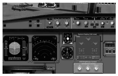
The System Display can now be viewed at its full. In addition the lower Panel shows the Standby-instruments for VOR and ADF, the Clock, the Dimmer for the displays, the Gear Lever display and the Autobrake panel.
