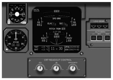
Here you'll find the complete System Display (SD). The SD displays Informationen for all the various aircraft systems. The displayed information changes automatically according to the actual flight situation.
