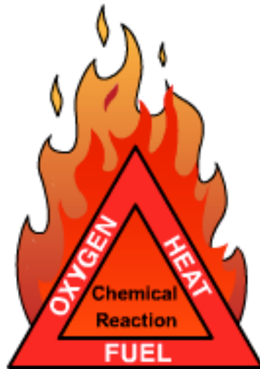
Figure 13 Oxygen Heat and Fuel Triangle
