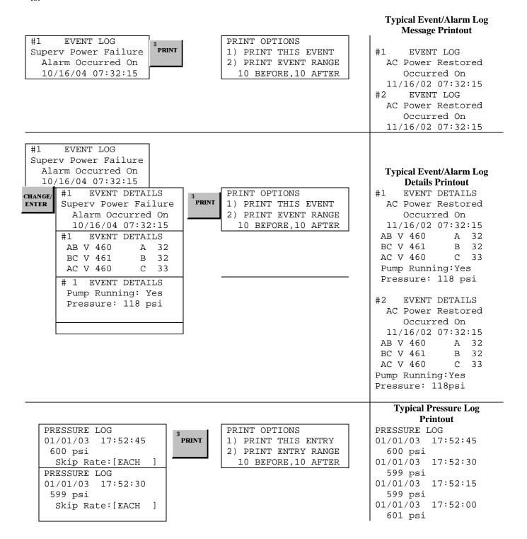
**CONFIGURATION SCREENS:** All parameters that control the operation of the controller can be viewed and changed within the Configuration set point screens. Each set point is protected by a user password to prevent unauthorized changes. The system set points are separated into five different group
