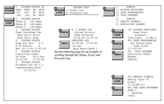
**SYSTEM LOGS:** The Model MP Electric controller has three separate data logs; 1) alarm log, 2) event log, and 3) pressure log. The alarm log is a subset of the event log and only displays the last ten alarms that have occurred or cleared. The event log records all alarm and system function type events
