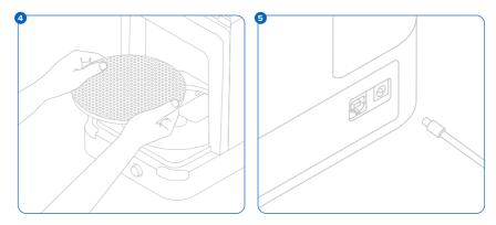
The Form Cure is ready to use once the turntable is installed and the power is connected. Each cycle requires time to preheat before the 405 nm lights begin post-curing. The preheating time depends on the current temperature and the target post-cure temperature.
