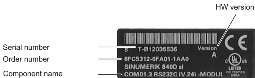
Figure 9-21 COM01.3 RS 232C (V.24) module type plate
