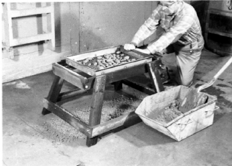
FIG. 5 Equipment for Wet Sieving Concrete by Hand
