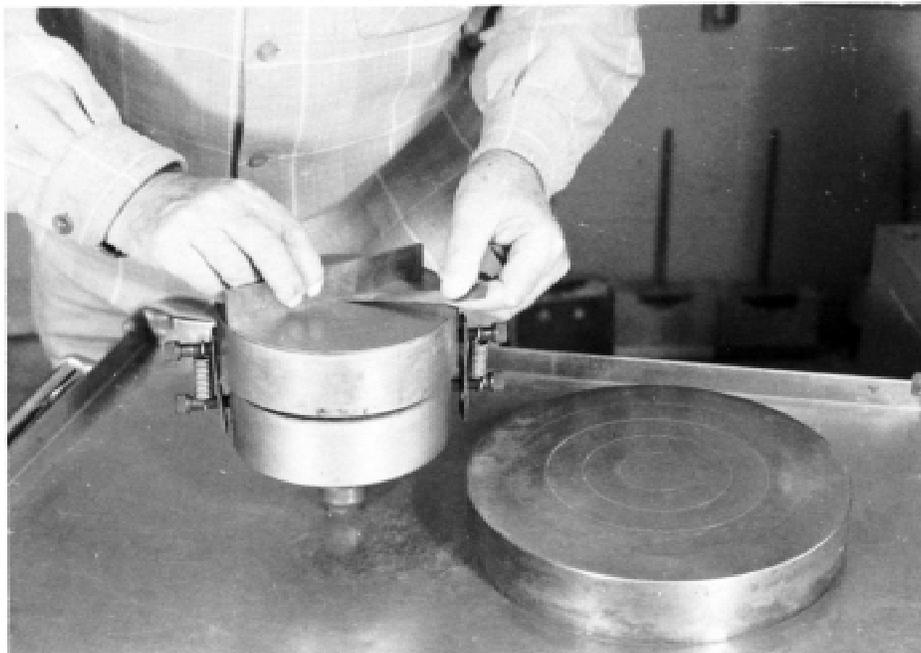
FIG. 4 Checking Planeness of Upper and Lower Bearing Blocks for a Testing Machine Using a Machinist's Parallel and a Feeler Gage of the Required Thickness
