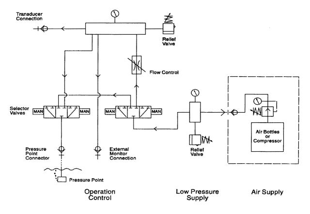
Figure 2.3 Schematic diagram of control equipment The air supply may be derived from high pressure air bottles or a compressor. Where a compressor is used the air receiver should be large enough to provide a supply for five days in the event of compressor breakdown or failure of the electricity supply.
