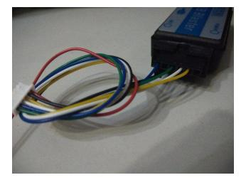
Note: this picture has a 12 pin connector, that's why the rightmost pins are not used. As you can see the wires are short. It's not recommended to build the cable with long wires as it has been found they won't work in some cases.
