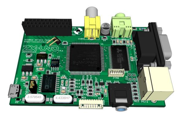
The ZX-Uno board is designed with same form factor than the original Raspberry Pi model A, having most of its connections placed at same place, allowing us to use boxes designed for that Raspberry Pi with minimal modifications.
