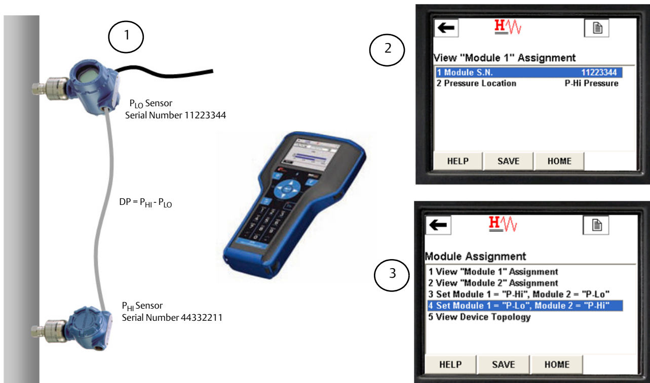
Figure 3-6. Example of How to Change the P HI and P LO Module Assignments
