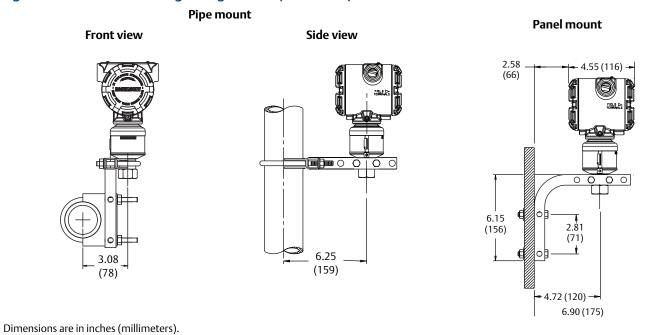
Figure A-11. Remote Display Mounting Configurations (B4 Bracket)
