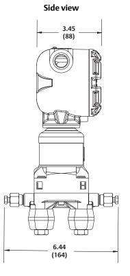
Figure A-4. Rosemount 3051S ERS Coplanar Sensor with Traditional Flange and PlantWeb Housing
