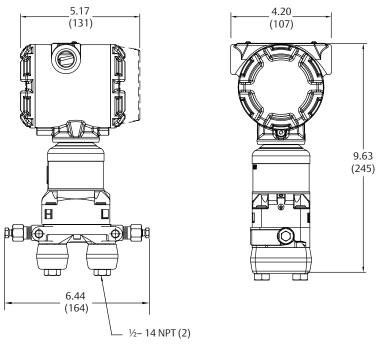
Figure A-13. Rosemount 3051S ERS Measurement Transmitter–In Line Style
