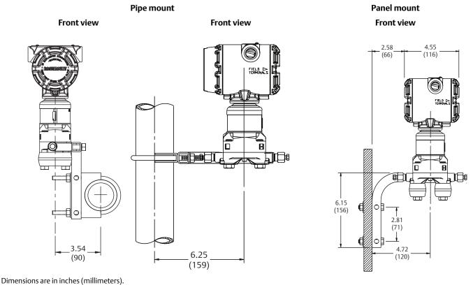
Figure A-9. Traditional Mounting Configurations
