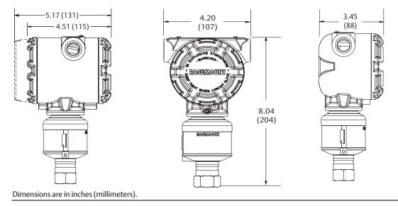
Figure A-14. Rosemount 3051S Scalable™ Level Transmitter with FF Seal<sup>(1)(2)</sup>
