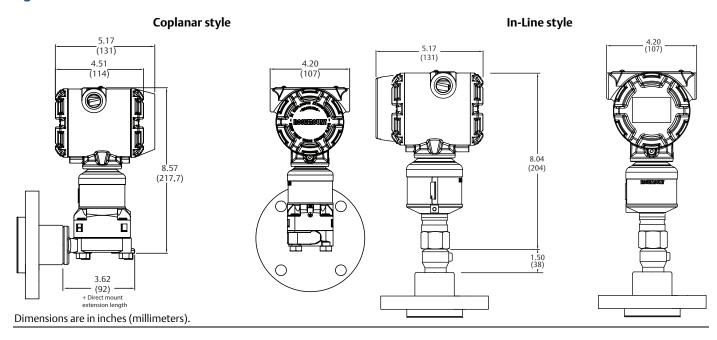
Figure A-15. Rosemount 3051S Scalable Level Transmitter with EF Seal(3)
