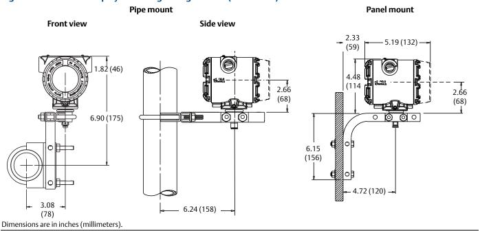
Figure A-12. Rosemount 3051S ERS Measurement Transmitter–Coplanar Style
