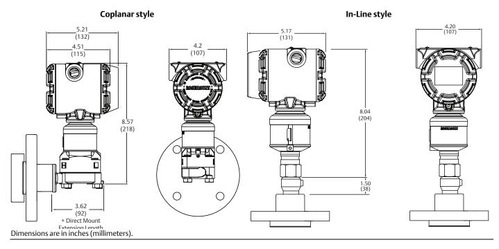
Figure A-17. Rosemount 3051S Scalable Level Transmitter with RT Seal<sup>(2)</sup>
