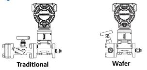
The Rosemount 306 Manifold assembles directly to an in-line style transmitter and is available with male or female  $^{1}/_{2}$ -in. NPT process connections.
