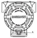
A. 23 Cover jam screw (1 per side) B. Cover jam screw
