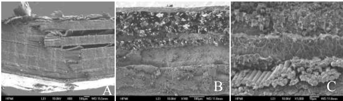
Figure 7. Three-point bending failure of random BP/CF hybrid exhibiting (a) delamination macro-scale failure, (b) visible layer differentiation of BP and CF, and brittle and (c) pullout failures of the CF and CNT
