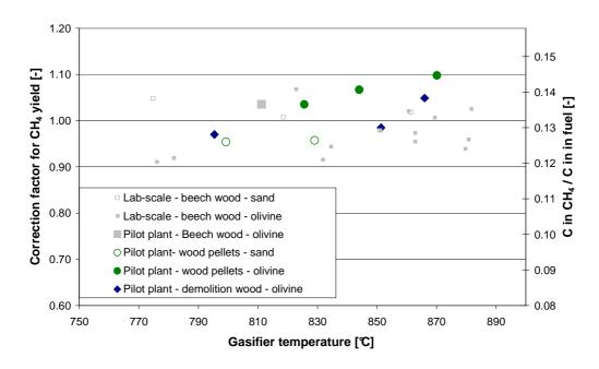
Figure 7-8: Correction for CH<sub>4</sub> yield as function of temperature.
