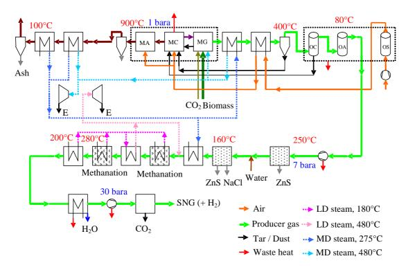
Figure 4-4: Scheme of Indirect gasifier SNG system.
