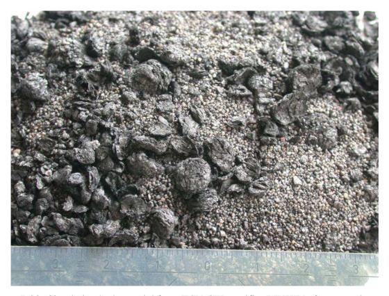
Figure 7-23: Circulating bed material from ECN CFB gasifier BIVKIN after test using wood pellets as fuel. Sand of 0.4-0.6 mm was used as original bed material.
