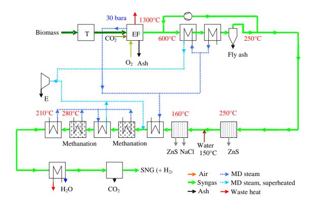
Figure 4-2: Scheme of EF SNG system.
