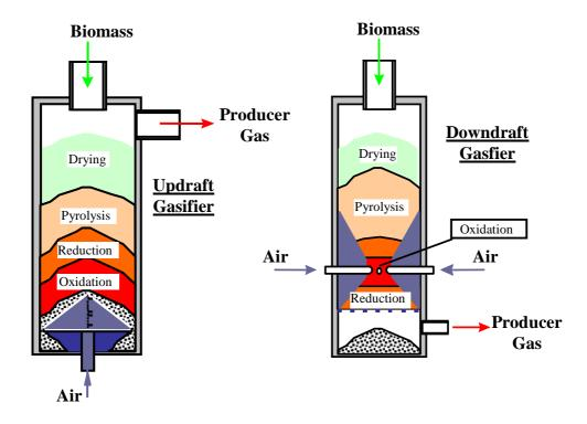
Figure 2-1: Schematic comparison of Updraft and Downdraft Gasification
