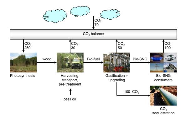
Figure 1-1: Indicative CO<sub>2</sub> balance for Bio-SNG system based on MILENA gasification.
