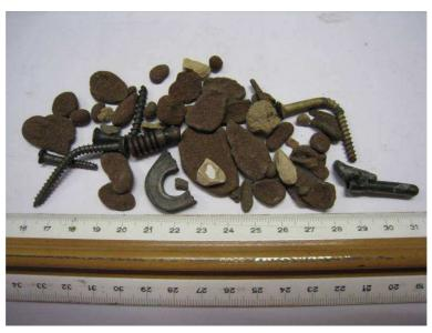
Figure 7-21: Typical example of ash particles discharged from riser.
