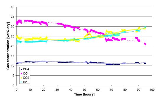
Figure 7-22: MILENA lab-scale duration test gas composition.
