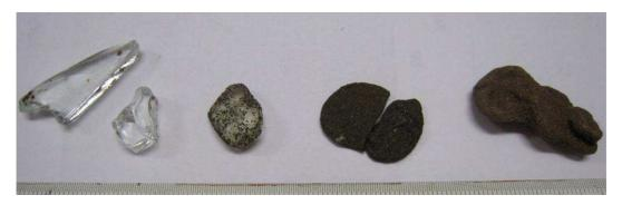
Figure 7-26: Various stages of bed material covering of glass particles.
