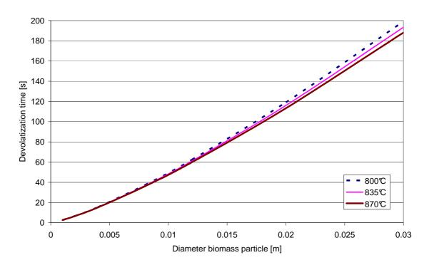
Figure 6-2: Calculated devolatization times assuming spherical particles.
