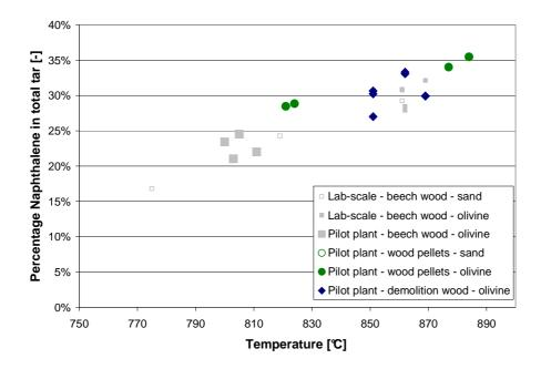
Figure 7-17: Mass fraction of Naphthalene in total tar as function of temperature
