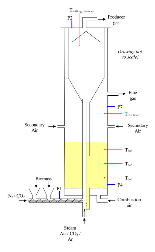
Figure 6-8: MILENA lab-scale gasifier.
