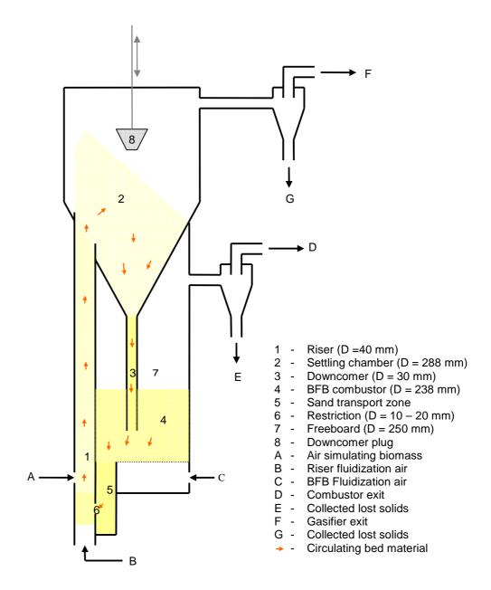
Figure 6-5: MILENA Cold Flow Set-up.
