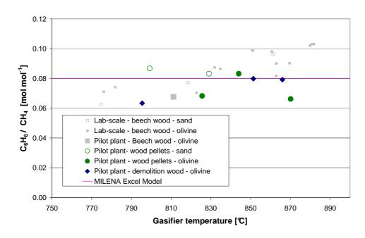
Figure 7-12: C<sub>6</sub>H<sub>6</sub> yield relative to CH<sub>4</sub> as function of temperature.
