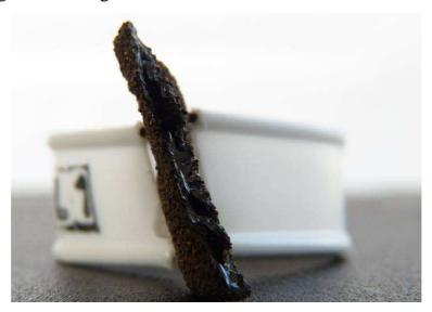
Figure 7-25: Close-up of broken glass particle.
