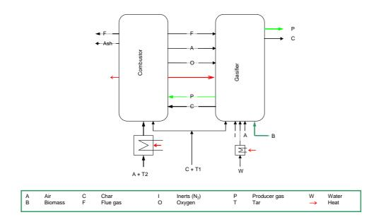
Figure 5-2: MILENA gasifier and combustor blocks.
