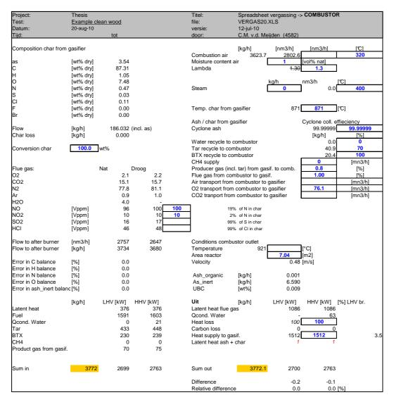
Figure 7-20: MILENA Excel model input and output for combustor.
