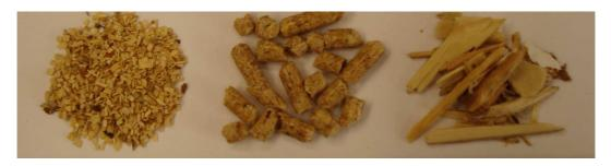
Figure 7-1: Beech wood, wood pellets and demolition wood as tested in MILENA gasifiers.
