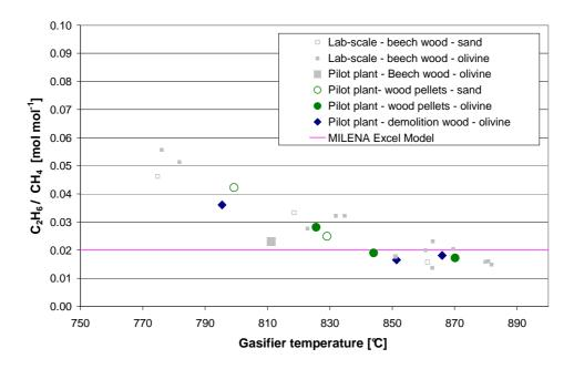
Figure 7-11: C<sub>2</sub>H<sub>6</sub> yield relative to CH<sub>4</sub> as function of temperature.
