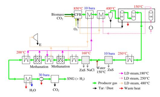
Figure 4-3: Scheme of CFB SNG system.
