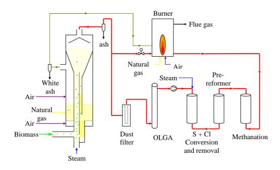
Figure 6-6: Basic layout of MILENA lab-scale installation.
