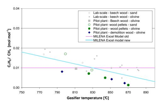
Figure 7-13: C<sub>7</sub>H<sub>8</sub> yield relative to CH<sub>4</sub> as function of temperature.
