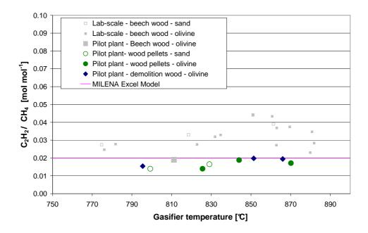
Figure 7-10: C<sub>2</sub>H<sub>2</sub> yield relative to CH<sub>4</sub> as function of temperature.
