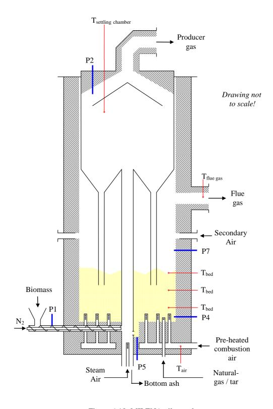
Figure 6-10: MILENA pilot-scale reactor
