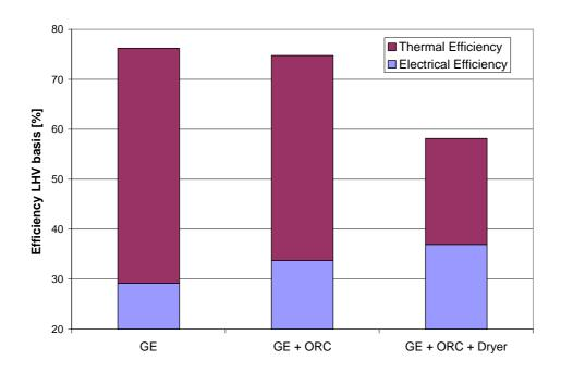
Figure 8-2: Calculated efficiencies of MILENA Bio-CHP configurations
