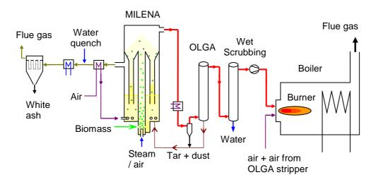
Figure 6-9: Basic layout of pilot plant
