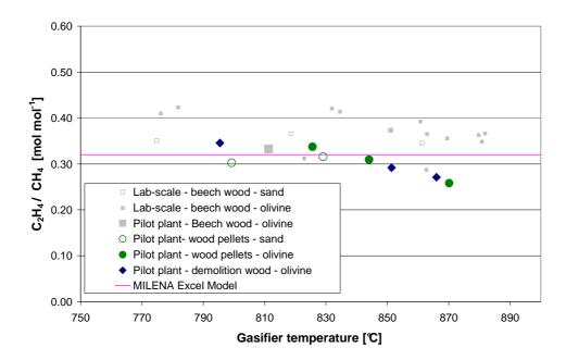
Figure 7-9: C<sub>2</sub>H<sub>4</sub> yield relative to CH<sub>4</sub> as function of temperature.
