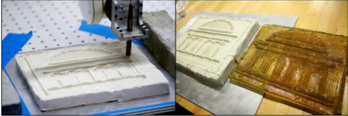
Figure 10. A Plasticine mold is sculpted by the robotic arm according to a design on the left (a) and a cast urethane part from the finished mold is seen on the right (b).
