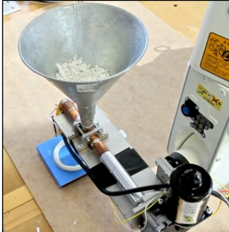
Figure 2. The HDPE 3D printing effector mounted to the robotic arm. Shredded HDPE plastic from recycled sources is fed into the hopper and extruded during printing.
