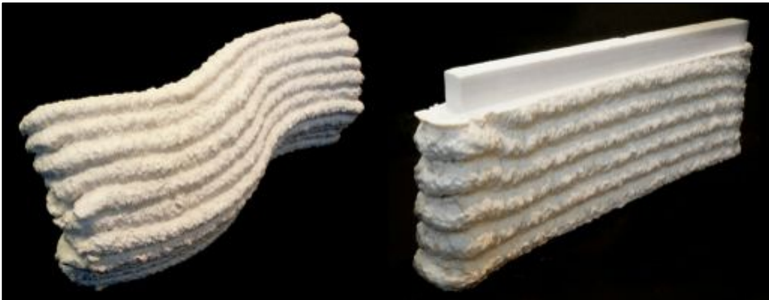
Figure 8. The urethane 3D printing system can print doubly curved structures as seen on the left (a) and the milling effector can be used to subtractively finish the foam according to a digital design as seen on the right (b).
