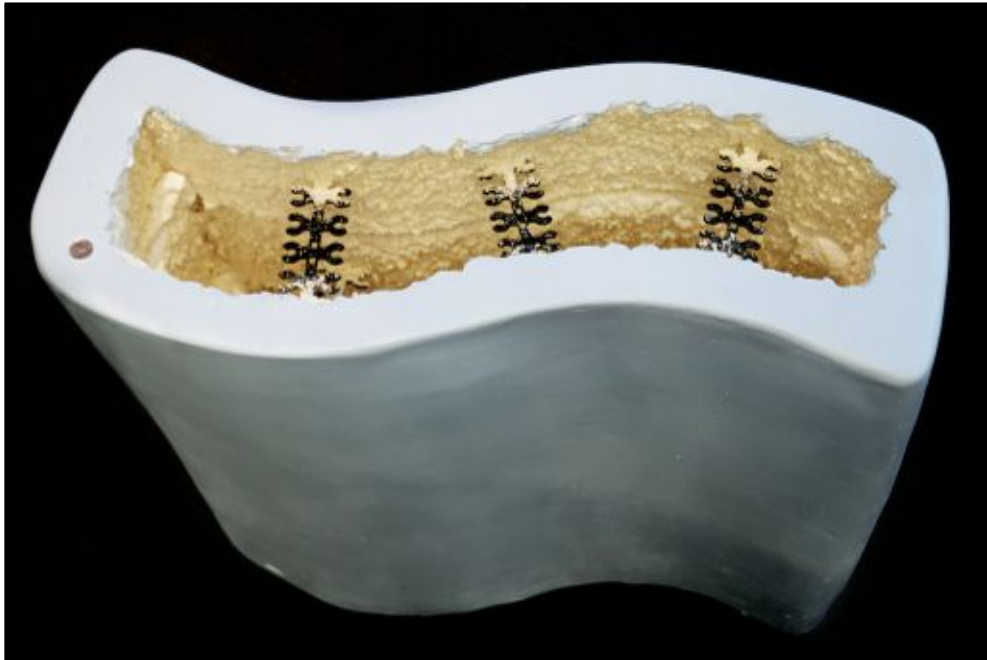
Figure 9. A 3D printed urethane foam wall mold with embedded plastic tie structures that has been milled and finished on the exterior with plaster and paint. This wall mold utilizes tie structures to support rebar during a concrete pour and the foam mold serves dual purpose as thermal insulation for the final wall. The wall structure is four feet tall and an American 25 cent coin is shown as a relative scale.
