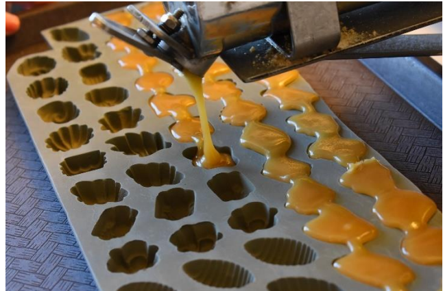
Figure 72 - Maple candy Maple candy being made with a commercial candy machine. (Image source Isselhardt, n.d.)
