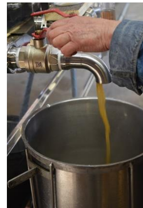
Figure 57 - Drawing off finished syrup from the evaporator (Image source UVM Extension, n.d.)
