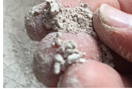
Figure 56 - Niter Image of niter that will build up on the bottom of the pan if not cleaned regularly (Image source Isselhardt, 2019)
