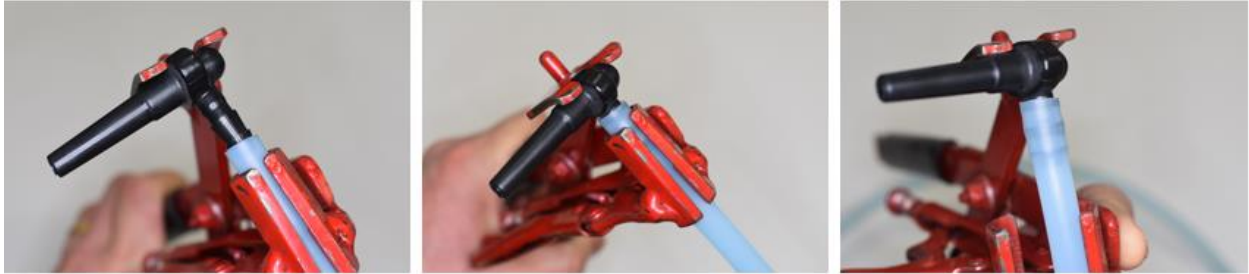
Figure 44 - Making a dropline Using a one-handed tubing tool to make a dropline. (Image source Isselhardt, 2019)
