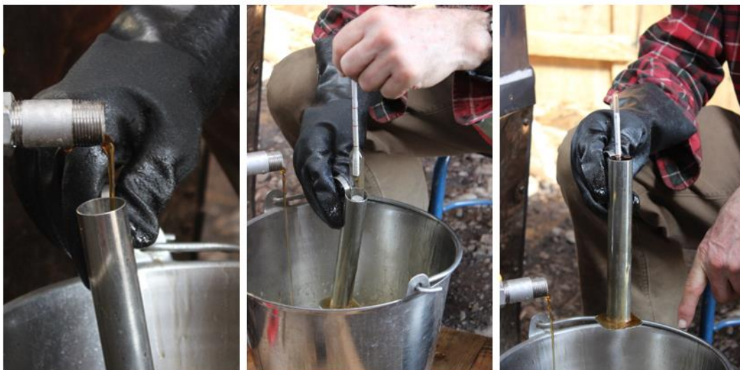
Figure 60 - Using a hydrometer Placing hydrometer in a hydrometer cup to test the density and determine if it is syrup. (Image source Shelburne Farms, n.d.)
