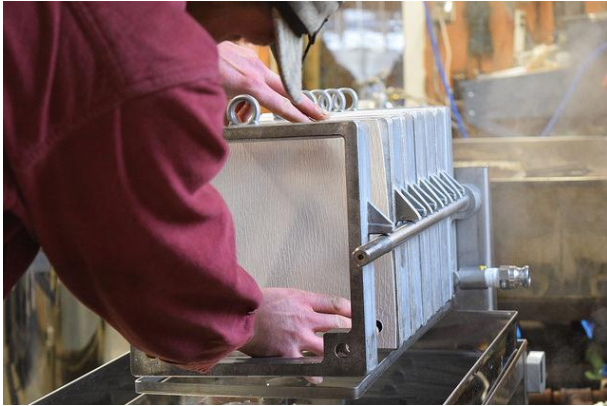
Figure 64 - Components of a plate filter press The components of a plate filter press include the filter press frame, end plates, filter paper, backer plates, and frame plates. Many of these components are visible in the photograph as a sugarmaker puts the filter press together in preparation of filtering a batch of syrup.
