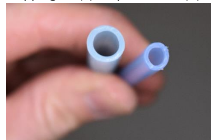
5/16" tubing (L) vs. 3/16" tubing (R)
