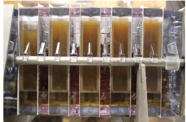
Figure 63 - Clear filter press When a filter press is constructed from clear material it is easy to view the filter compartments and the filtering DE "cakes" that form in the frame plates. (Image source Shelburne Farms, n.d.)
