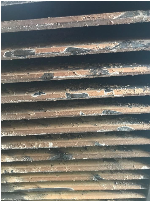
Figure 31. Flues on underside of sap pan showing dark areas where holes were found
