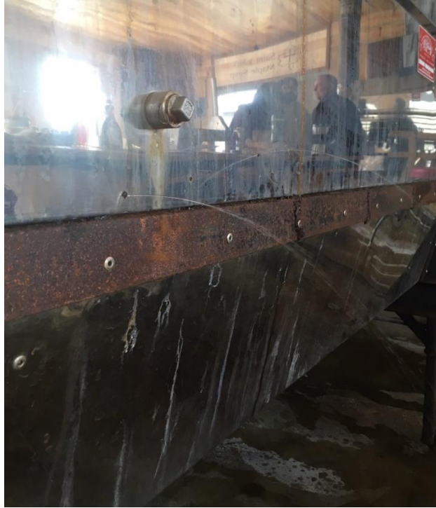
Figure 30. Sap pan with two leaks shooting a fountain of sap
