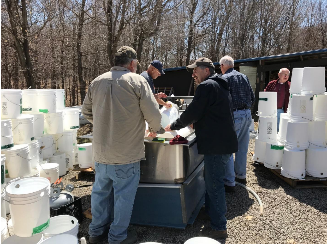
Figure 17. Bucket washing station. The stainless steel tank is filled with hot soapy water. It is kept hot by a heater placed beneath the unit. Sheet of tin surround the bottom of tank to keep the heat focused on the tank. Jim Preusser (foreground) hands pails to a prewasher (Mark Ludowese, right foreground) who does a quick scrub and then passes the bucket to Bill Mock (left) and Dan Weber who do the final cleaning on a rotating drum.
