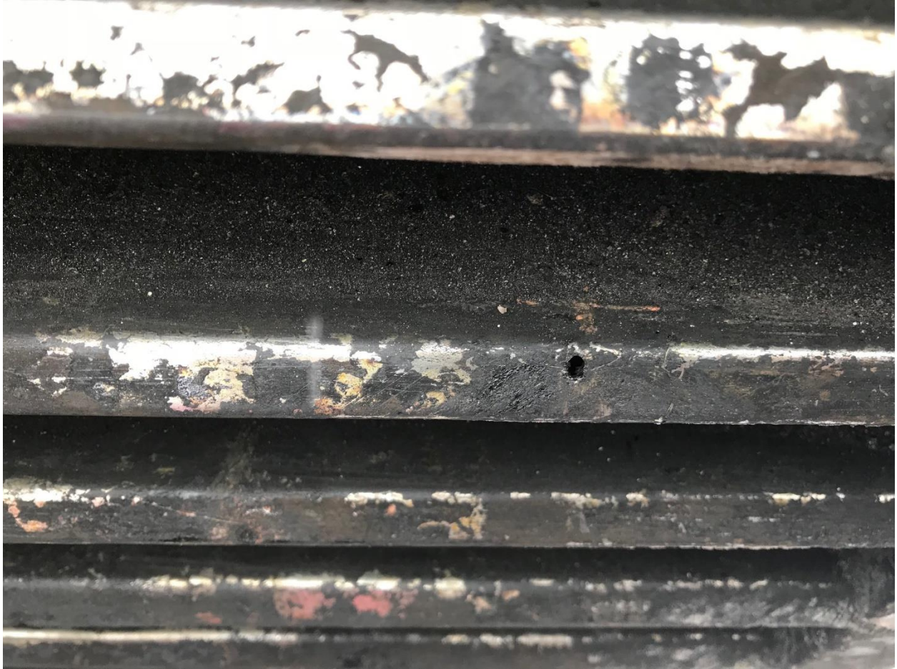
Figure 32. Close-up view of hole in a flue of the sap pan. This hole is approximately the diameter of a pencil.
