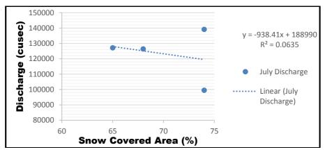
**Figure 8:** Discharge rate with respect to snow covered area in the month of July in the melting period from years 2004-2017
