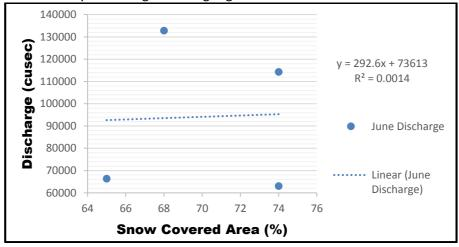
**Figure 7:** Discharge rate with respect to snow covered area in the month of June in the melting period from years 2004-2017
