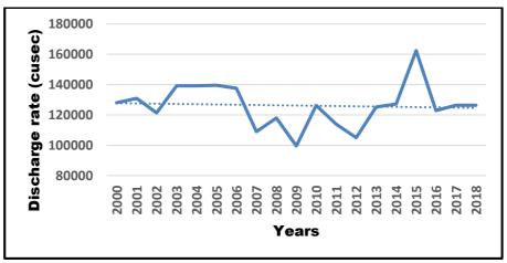
**Figure 6:** Discharge rate changing with the passage of time in the month of July from 2000-2018
