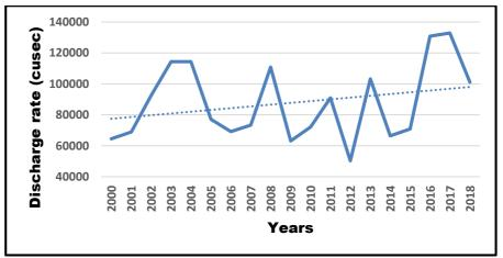
**Figure 5:** Discharge rate changing with the passage of time in the month of June from 2000-2018
