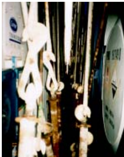
Insufficient access in between container lashings (shown is only 200mm)
