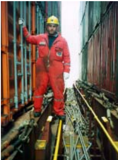
BEFORE - No consideration given to access. Vessel securing plan dictates three-high lashing which is not safe from this position, particularly when wet or icy.
