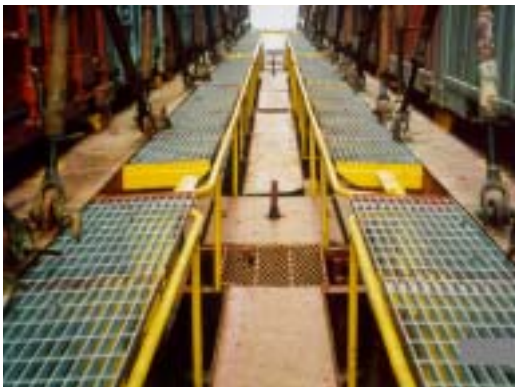
AFTER - Same vessel after modifications. Now safer enabling improved lashing efficiency and improved 'turn round' times in port.
