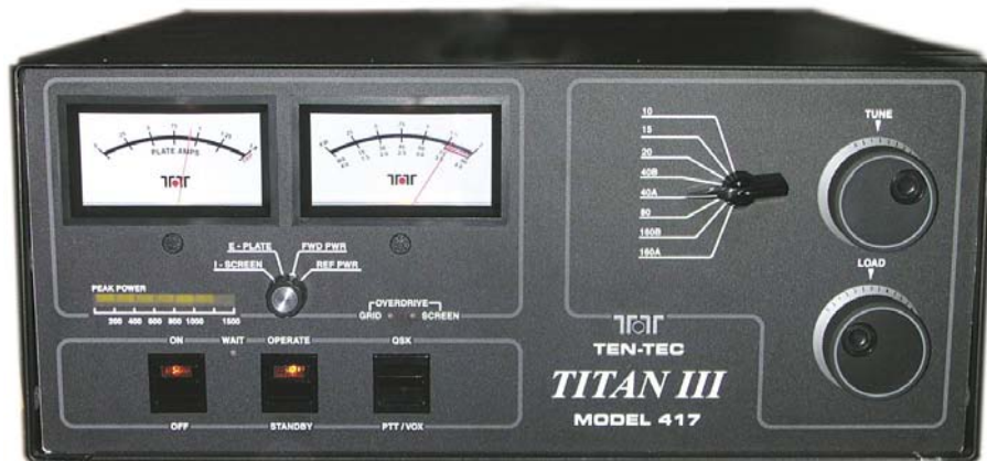
Figure 1—Front view of the Ten-Tec Titan III while it is pumping out 1500 W.
