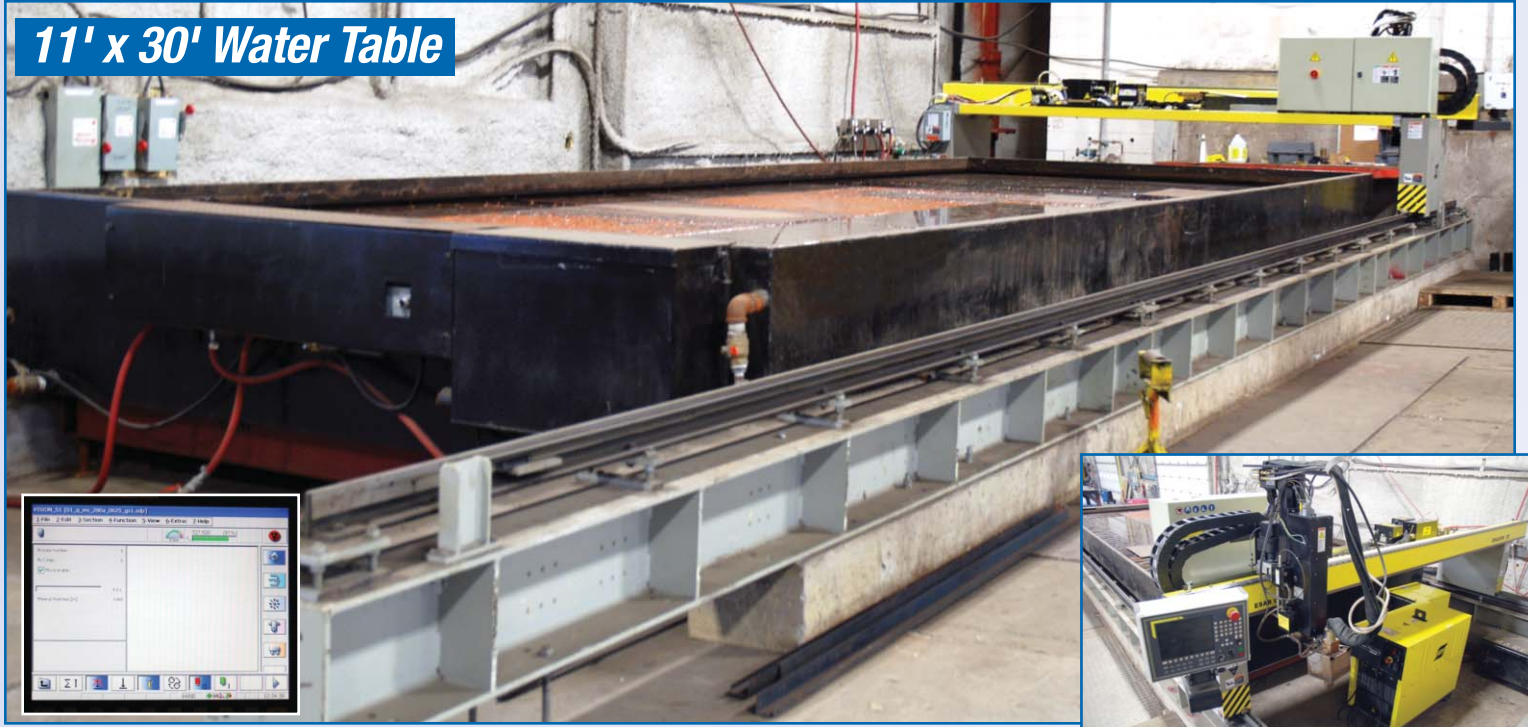
ESAB Shadow Dx-4000 Gantry Type Plasma Cutting System With Precision Plasmart 360 Power Source, CC-11 Coolant Circulator, Up To 2" Cutting Capacity, Note: Low Hours S/N 0560947520
