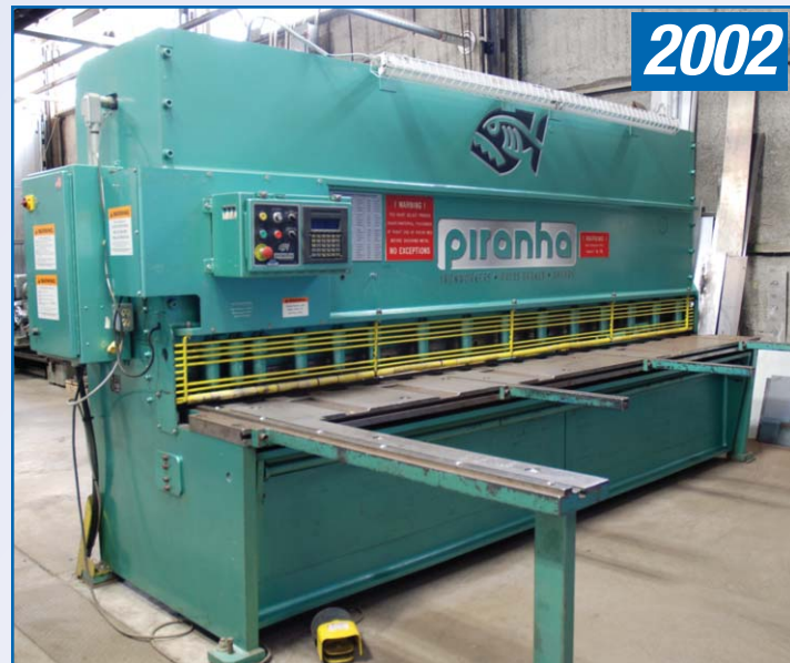
PIRANHA Model TC3/8-12, 3/8" x 12ft Hydraulic Shear With CNC Full Programmable Back Gaugefront, 24 SPM, 15 Holddowns, 20 HP, 24 500 Lbs, 49" Squaring Arm, (3) 24" Support Arms, S/N T3/8-12-1002
