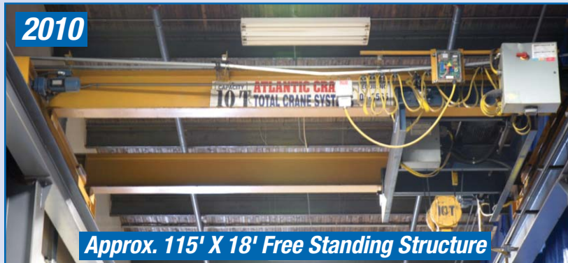
ATLANTIC CRANE 10 Ton Overhead Bridge Crane, Top Running, Double Girder, Approx. 18ft Span, 10 Ton Hoist, Buss Bar, Top Running Rails, I-Beams, Remote Control
