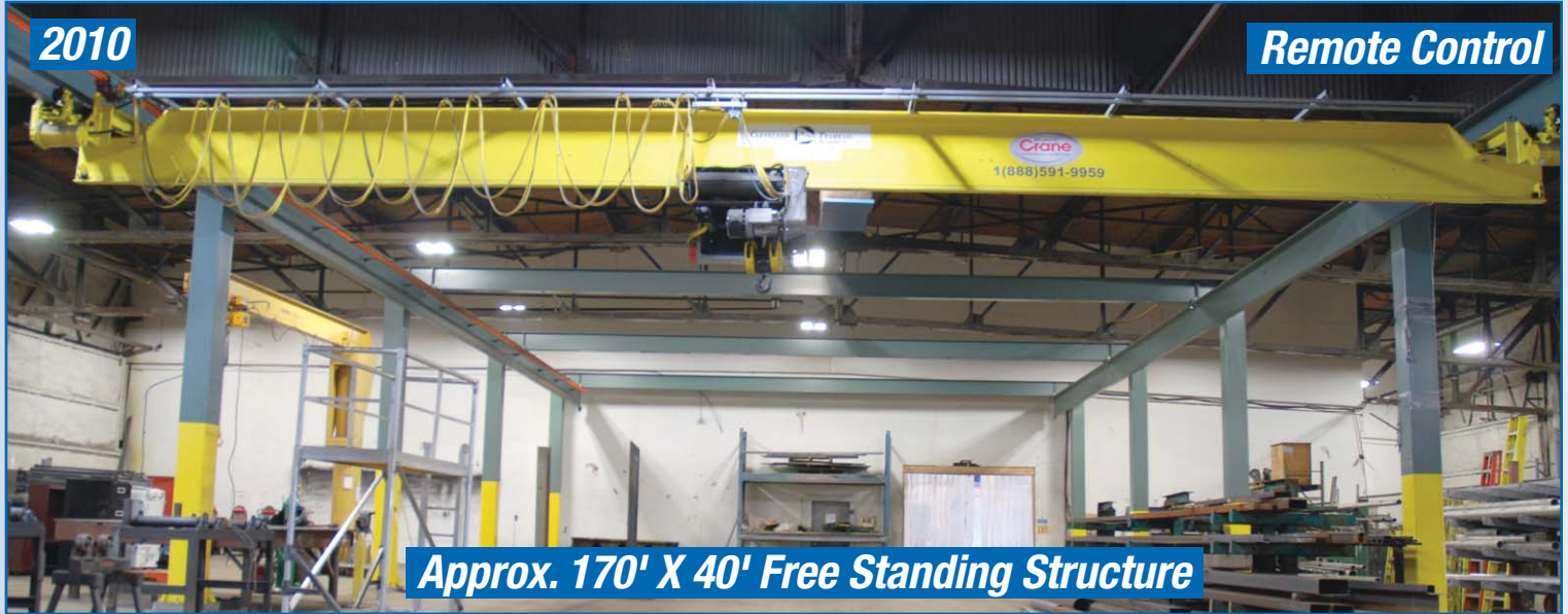
ATLANTIC CRANE 15 Ton Overhead Bridge Crane, Underslung, Single Girder, Approx. 40ft Span, 15 Ton Underslung Hoist, Buss Bar, Top Running Rails, I-Beams
