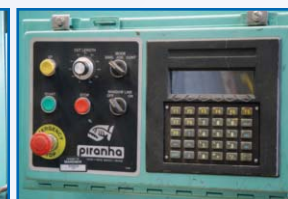
PIRANHA Model TC3/8-12, 3/8" x 12ft Hydraulic Shear With CNC Full Programmable Back Gaugefront, 24 SPM, 15 Holddowns, 20 HP, 24 500 Lbs, 49" Squaring Arm, (3) 24" Support Arms, S/N T3/8-12-1002
