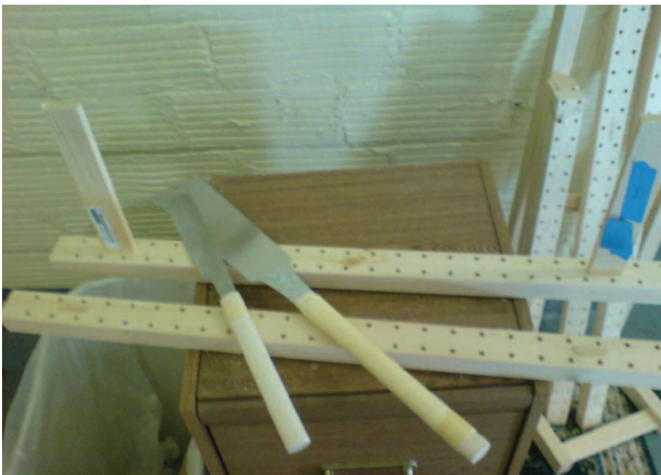
My father-in-law gave me these awesome nokogiri Japanese saws. The Ivar side trusses are glued and stapled together. I worried about hitting a staple with the saw, but they were avoidable or removable. [image: greg.org]
