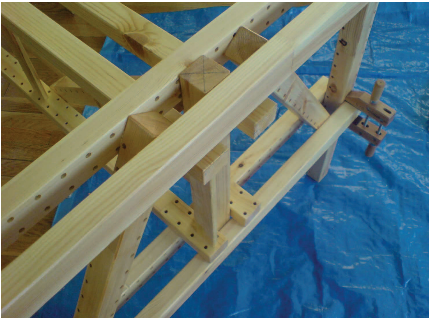
Test assembly of the table's three structural elements, originally for marking bolt holes. That clamp is holding together a split repair which I made with my first nail. [image: greg.org]
