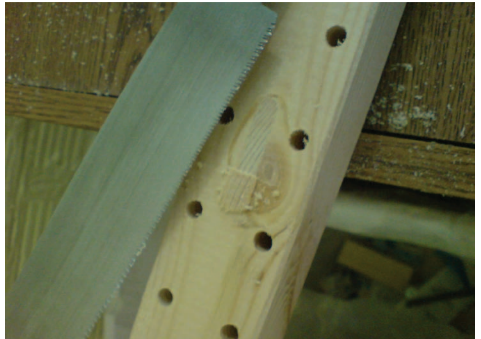
Nokogiri: cutting flush with a Japanese joinery saw. [image: greg.org]
