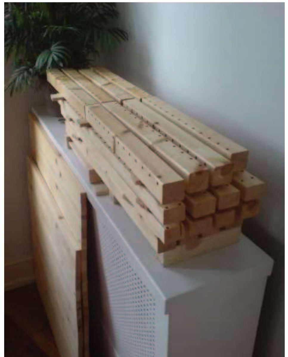
Tung oil varnish curing after 2nd coat. [image: greg.org]
