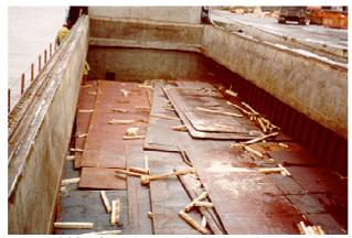
Shift of Inadequately Secured Cargo
