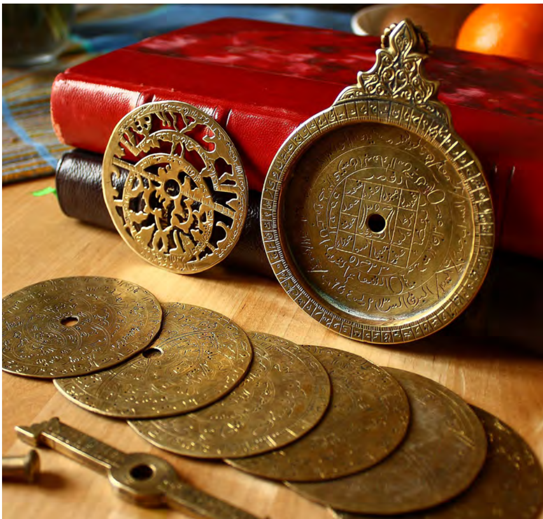
The various parts of a 18th century astrolabe, disassembled made in North Africa.
