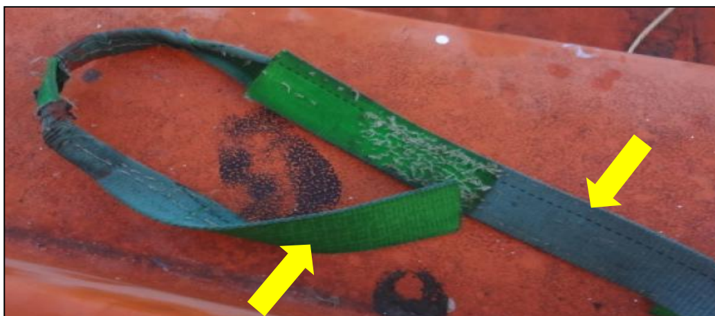
Figure 6: Failed section exposed to sunlight
