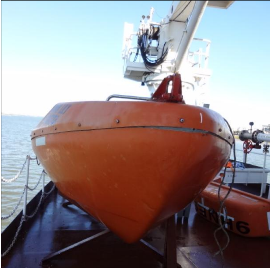
Figure 4: Davit/crane for launching rescue boat
