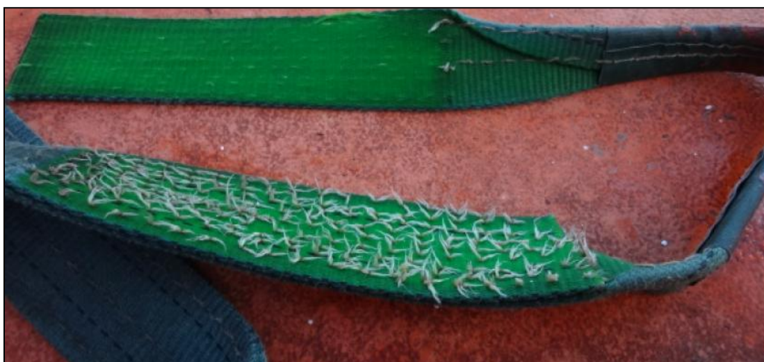
Figure 5: Failed section of the forward lifting sling
