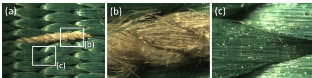
Figure 4 Optical micrographs of relatively undamaged regions of the sling.
