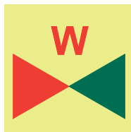
7132W Fire main section valve PP
