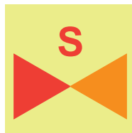
7132S Sprinkler section valve PP
