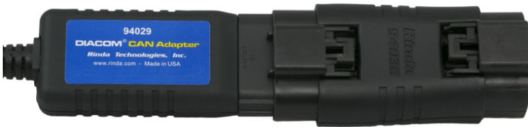
Figure 24 Adapter #94029 attached to #94032
