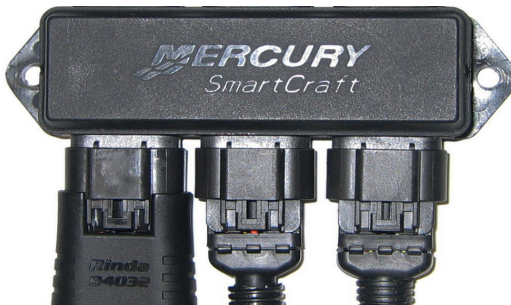
Figure 25 Adapter #94032 attached to junction box
