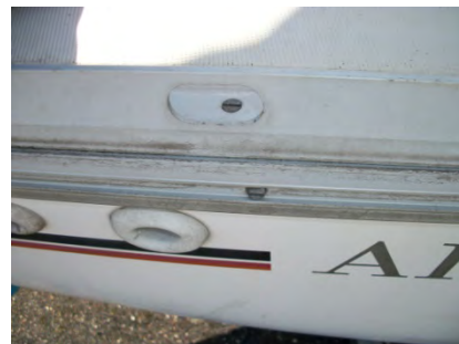
Fig 14 Toe rail fixings external
