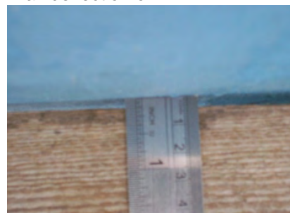
Fig 4 Detail of hull deflection
