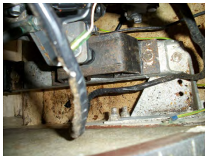
Fig 39 Loose wiring in engine
