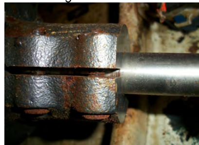
Fig 21 Detail of shaft in coupling has spun in the past in the Fenwick
