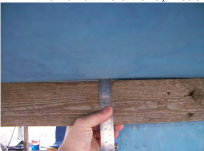
Fig 3 Area of hull deflection
