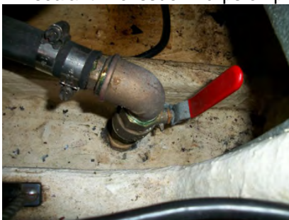
Fig 22 Engine intake. Suggest laminate nut to hull. Page 13 of 13
