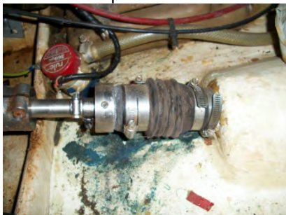
Fig 20 PSS Stern Gland and seal
