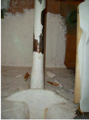
Fig 19 Signs of surface rust on rudder tube
