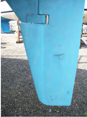
Fig 17 Rudder from port side clearly showing a line of weeping
