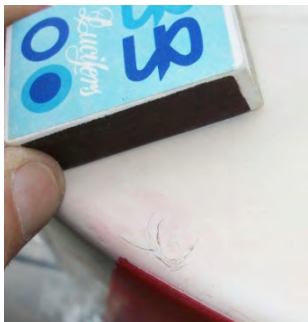
Fig 7 Gel coat damage on transom
