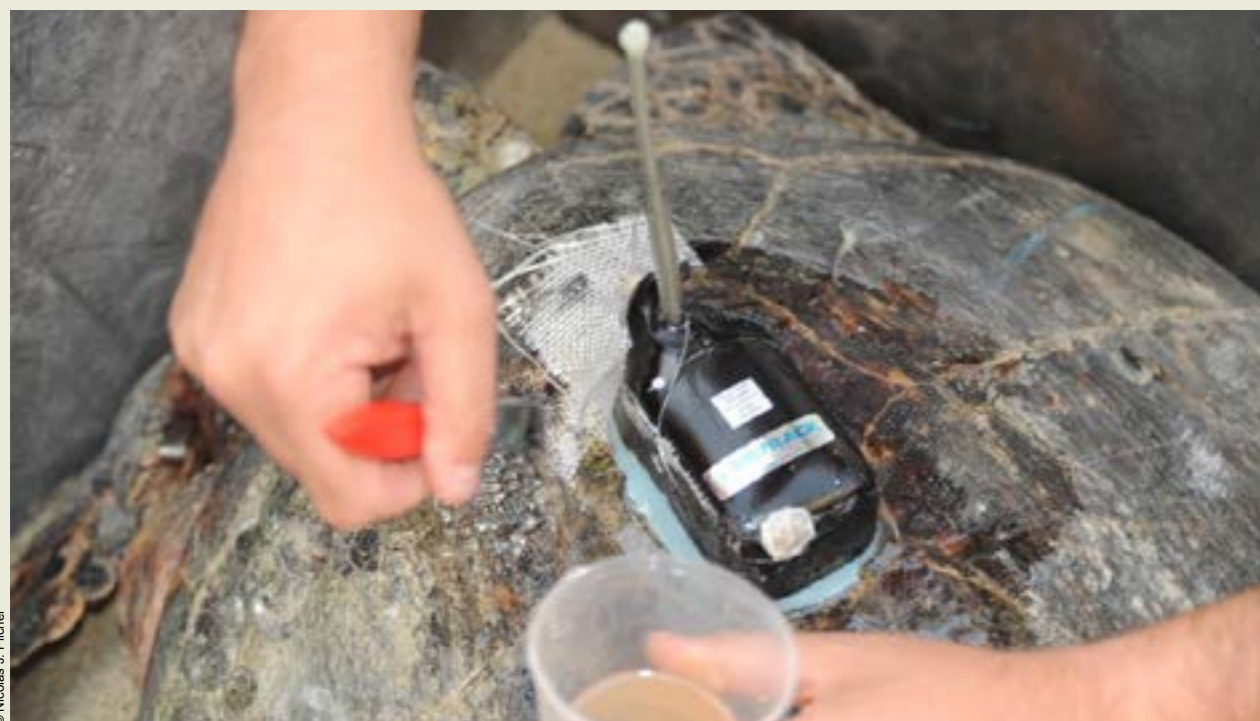
Figure 6: PTT being affixed on top of the turtle carapace using fibreglass cloth and resin.
