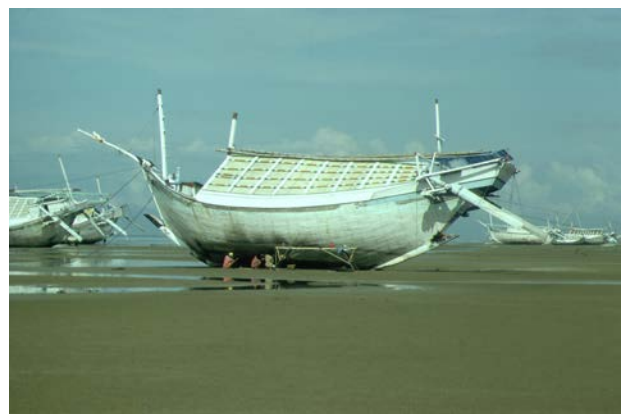
A big fat janggolan being recaulked on the beach at low tide.
