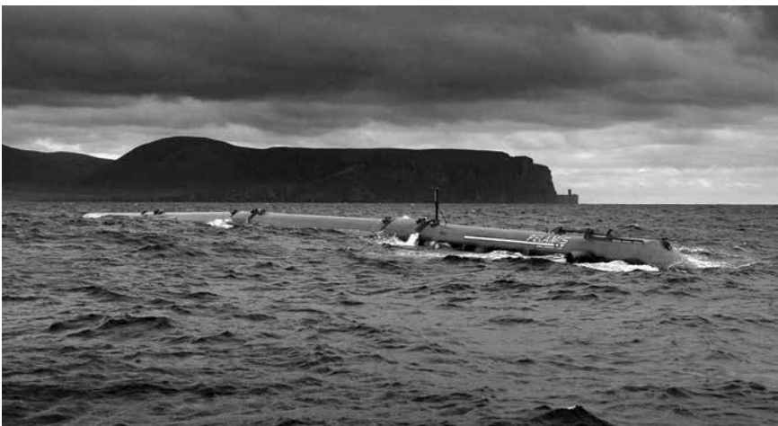
Figure 5.2. The Pelamis Wave Power prototype. Source: Wikimedia Commons.
