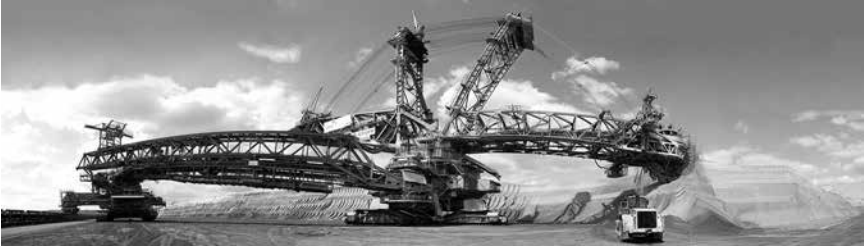
Figure 2.2. New mining technology often involves very large equipment. Bagger 288, a mobile strip-mining machine, is the world's largest land vehicle. Source: http://commons.wikimedia.org/wiki/File%3ABagger-garzweiler.jpg
