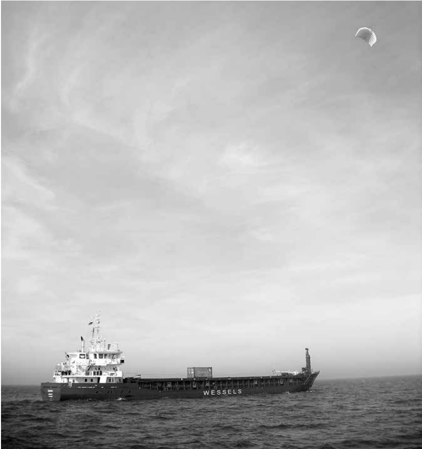
Figure 5.5. The cargo ship MV Theseus fitted with an aerial kite. Credit: “ Theseus-Quelle WesselsReederei ” by Reederei Wessels - Reederei Wessels/Fotoflite. Licensed under CC BY-SA 2.5 via Wikimedia Commons - http://commons.wikimedia.org/wiki/File:Theseus-Quelle_WesselsReederei.jpg#/media/File:Theseus-Quelle_WesselsReederei.jpg
