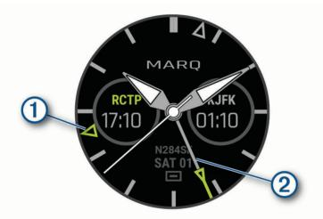
① Alternate time zone pointer. References the 24-hour time markings on the watch, in up to four alternate time zones (Adding Alternate Time Zones, page 73).
