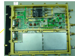
Filtering and Switching Unit
