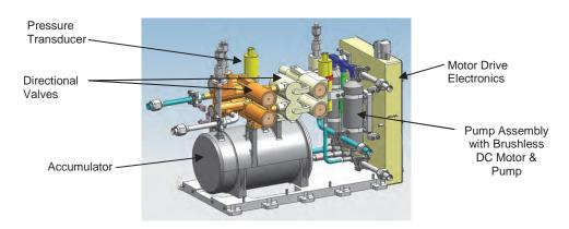
Figure 4. Rover Integrated Pump Assembly (RIPA)
