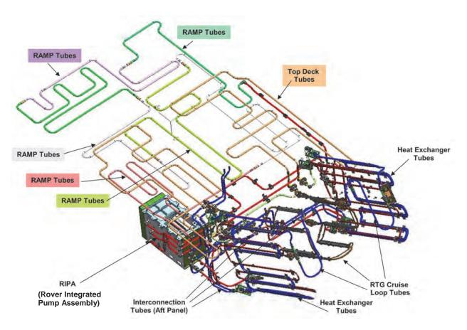
Figure 2. Heat Transfer System of Piping in the Rover and Around the RTG
