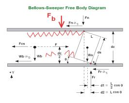
Figure 10. Free Body diagram of bellows assembly in housing
