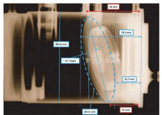
Figure 7. Measurements made using the X-ray of the Accumulator Assembly
