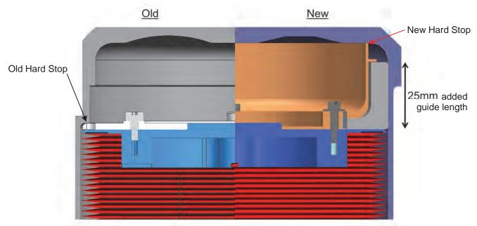
Figure 14. Original and Final designs of the end of the bellows assembly. The figure shows the bellows stroked to the maximum fluid condition and against the end-of-stroke hard stop for both design versions
