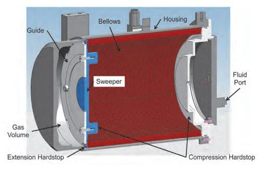
Figure 5. Accumulator Assembly showing bellows in fully extended position (maximum fluid volume, maximum pressure of gas)
