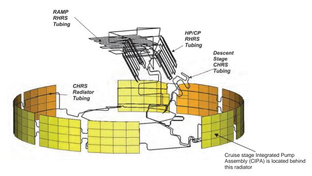
Figure 3. Heat Transfer System of Piping in the Cruise Stage and Relationship to the Rover System of Piping
