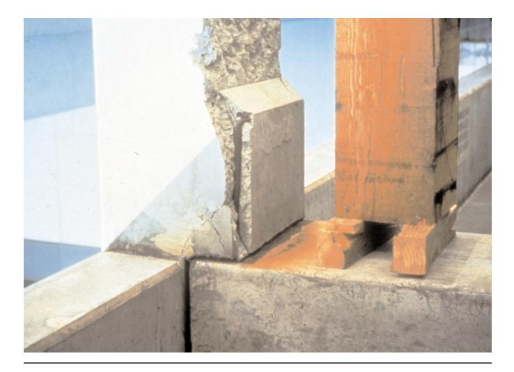
In this slide we can see a rebar anchor that had been placed too close to the edge. Location is critical to rebar performing as it should during an earthquake. When it is too close to the edge, as here, it won't be able to provide the necessary confinement for the concrete. The placement of rebar is very important. Even small deviations in rebar location can significantly reduce concrete's strength and ductility.
