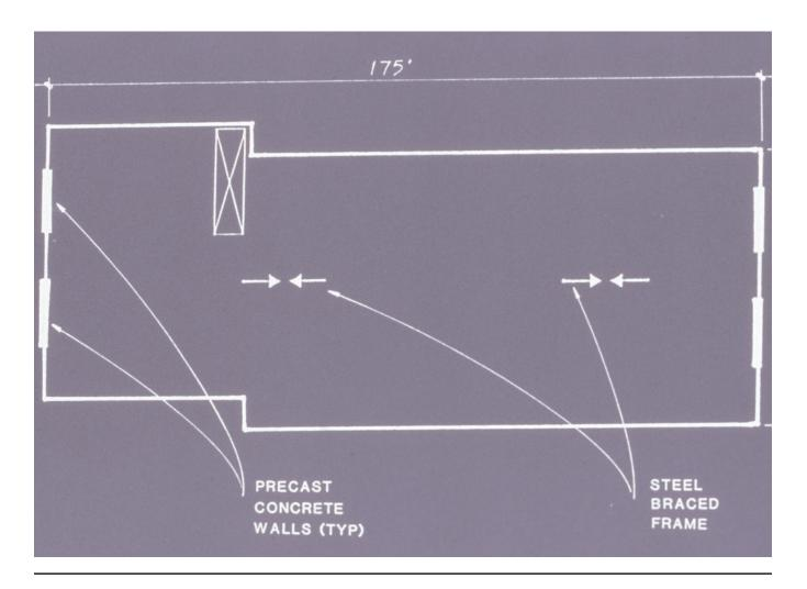
This is a floor plan of the building. You can see that the lateral system for the building in the short dimension direction, also called the transverse direction, consists of concrete shear walls at both ends of the building.
