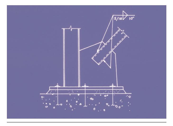
This is a connection detail drawing showing a correct weld symbol for both side welding of a brace to a gusset plate.
