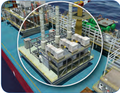
Intermediate - Pressure Gas - Lift Compressors
