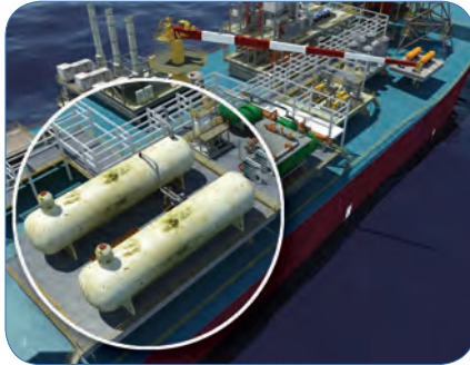
Crude Oil Treatment, Desalting
