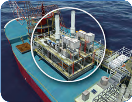
High - Pressure Gas - Injection Compressors
