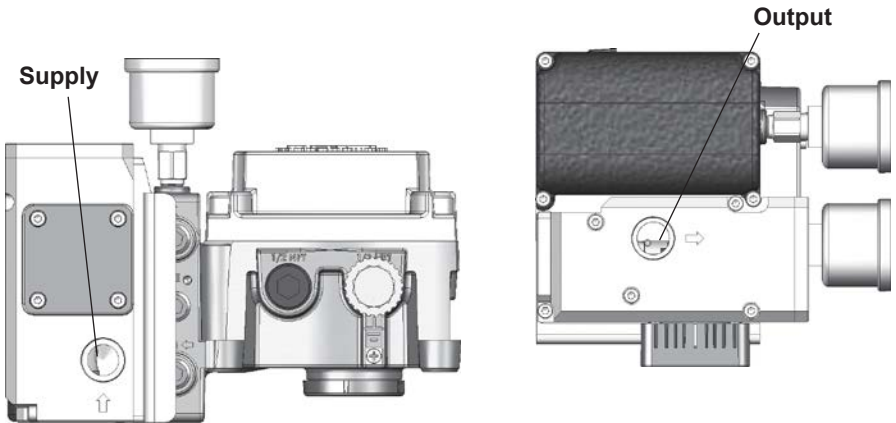
Figure 5 - SVI II AP High Flow Air Ports on Single Acting Positioner
